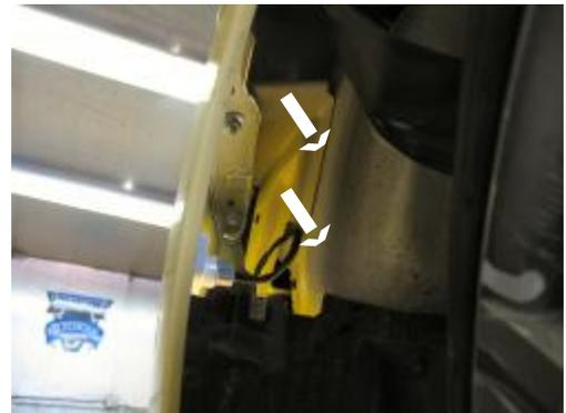
4. Forward of front tires is a metric hex nut to remove and one metric bolt to loosen with the 10MM socket, on both sides.
