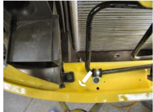
8. Remove the push pin from the back side of metal bumper, on both sides, remove air dam and set aside.
