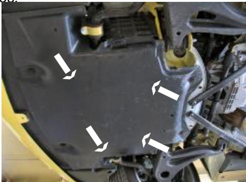
5. Remove the four metric bolts from the belly pan using the 8MM socket, release the two clips on the sides of belly pan, set aside.
