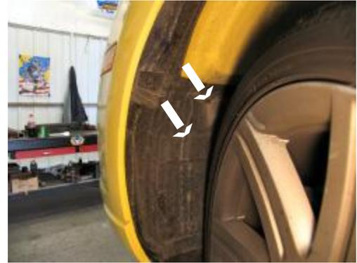
2. Just forward of front fascia on wheel well edge are two Torx screws to remove with the 30 Torx socket, on both sides.
