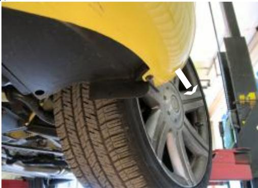
3. Just forward of front tire is a Torx screw. Remove with the 30 Torx socket, on both sides.
