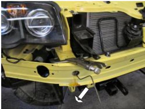
9. Slide baseplate between frame rails just behind metal bumper and clamp to frame with the large vise grip, on both sides. **Be sure that baseplate is level with vehicle.**
