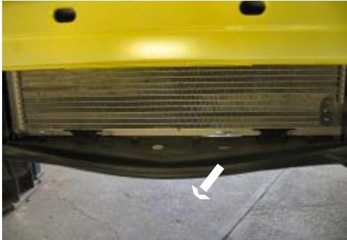
7. Remove the four push pins from air dam just below bottom edge of radiator.
