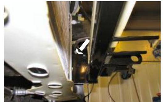
10. Using the baseplate as a template, drill the three holes into the frame with the 13/32" drill bit, on both sides. Insert the nut plates into the opening on the front side of metal bumper (See white arrow in step 9) to align with drill holes, tighten the lock washers and 3/8-16 x 1 1/4" hex bolts with the 9/16" socket, on both sides. **Be sure to use Loctite red on all bolts before tightening. Tighten all bolts according to torque chart in the General Instruction sheet.**
