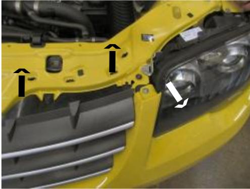
1. Remove the two metric bolts from top side of upper grill edge with the 8MM socket (white arrows), both sides. Using the 30 Torx socket, remove the Torx head screw (black arrow), on both sides.
